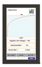
In the charge decay method, an electrode placed on the material under test and in contact with its surface is charged to a specific test voltage. The time required for the electrode to discharge to one of two pre-set limits (default - 50% or 10%), is then measured
